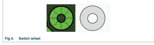
The switch wheel is implemented as eight interleaved pairs of sensor pads connected to eight sensor channels.
