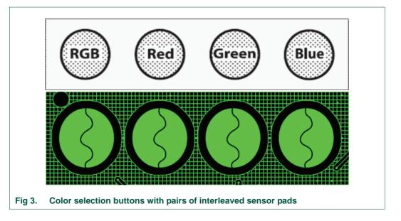
As shown in <u>Figure 3</u>, the buttons for color selection are made of two interleaved sensor pads connected to two separate sensor channels. In order to make sure that both channels are activated, the touch should be centered on the graphical icon engraved on the acrylic overlay.
