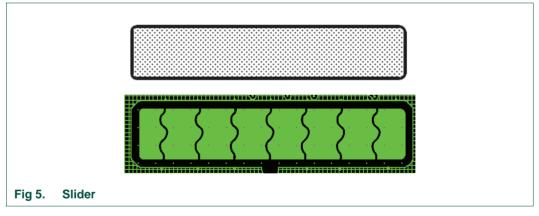
The slider is implemented as seven interleaved pairs of sensor pads connected to eight sensor channels.
